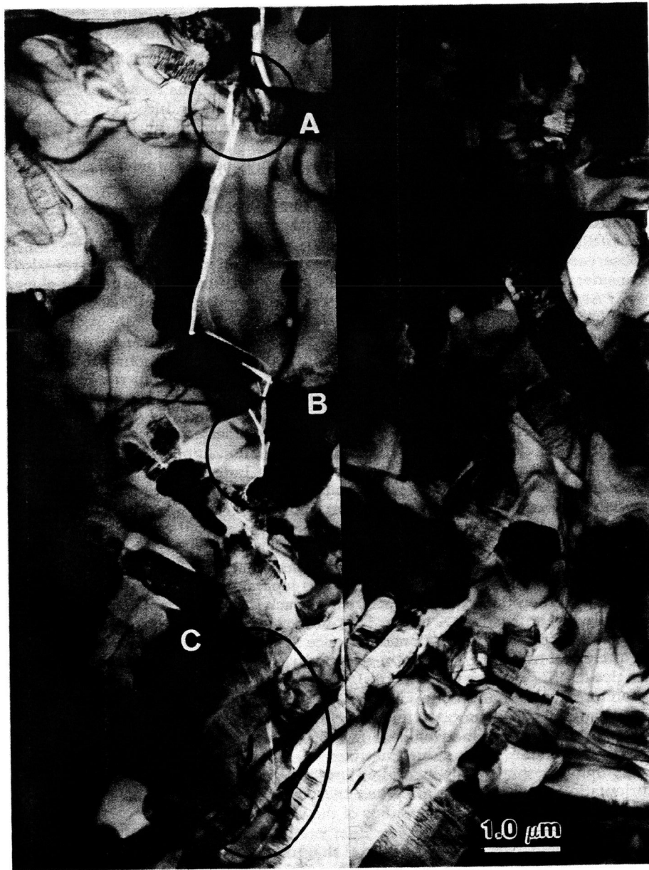
Fig 1. A TEM micrograph, of SiC/Al 2 O 3 composite, near a Vickers indent. The crack path is clearly visible, and the crack tip is indicated by an arrow. Region A shows that the whisker fracture occurs normal to the whisker axis. Region B indicates that fracture in the alumina matrix occurs along grain boundaries. Region C describes the bridging zone near the crack tip.
