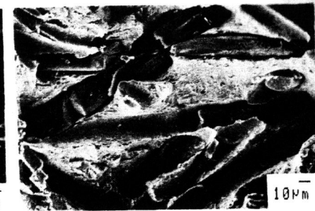
Fig. 6 Fracture surfaces at 600°C, vacuum a) as HIP IC-218 b) IC-218/Al 2 O 3 .
