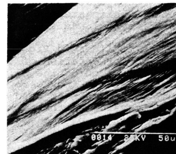
Fig.3. Slip structure in shear band of GP1-1.
