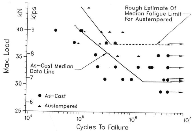
Fig. 8 Superposition of load versus cycles, as-cast and austempered
