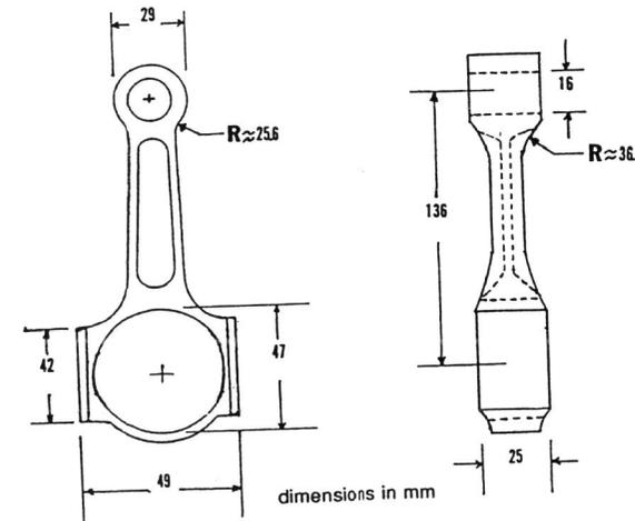
Fig. 2 Connecting rod test specimen
