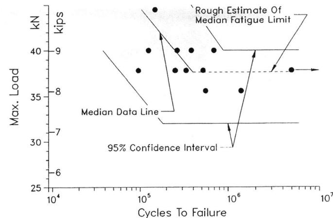
Fig. 4 Load versus cycles, austempered
