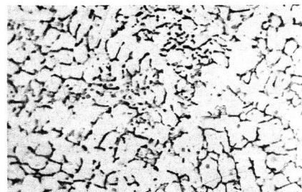
Fig. 8b. Micro-structure of weld metal exposed to 800°C. (X 1000 ).
