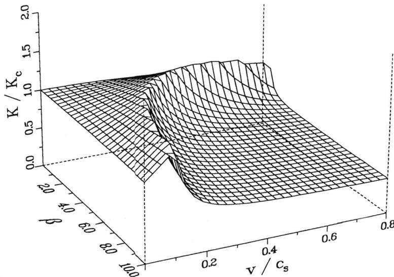
Fig. 6. Dependence of the applied dynamic stress intensity factor on crack speed  $v$  and viscosity parameter  $\beta$  implied by the condition that either a critical crack tip opening displacement growth criterion or a critical stress criterion can be satisfied by the material, with the choice determined by whichever can be satisfied by the lower level of  $K$ .
