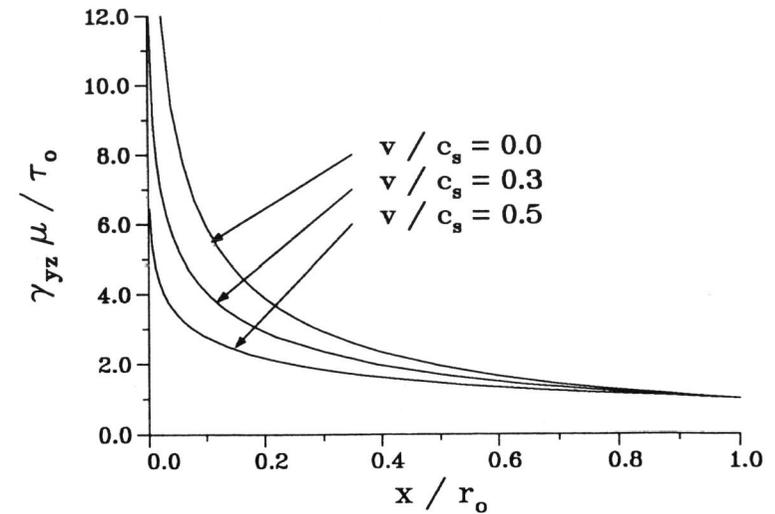
Fig. 1. Strain on the crack line in the active plastic zone for steady dynamic growth of a mode III crack in an elastic-ideally plastic material from (3).
