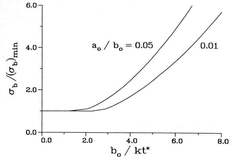
Fig. 3. The stress required to expand a thick spherical ideally plastic shell to a specified size versus the time required to do so for two values of initial hole size.
