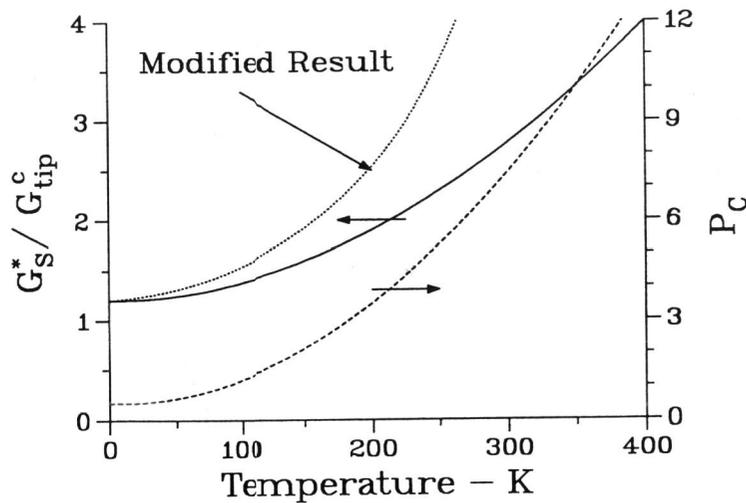
Fig. 5. The minimum driving force  $G_S^*$  needed to drive the crack dynamically as a function of temperature. The solid line results from Fig. 4, and the dashed line from a modified result due to Mataga et al (1987).
