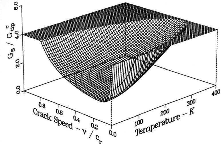
Fig. 4. A surface representing conditions on applied crack tip driving force  $G_S$ , crack tip speed  $v$  and temperature that correspond to steady crack propagation, as predicted by (14). The plateau is an artifact arising from truncation of the surface at a suitable level.
