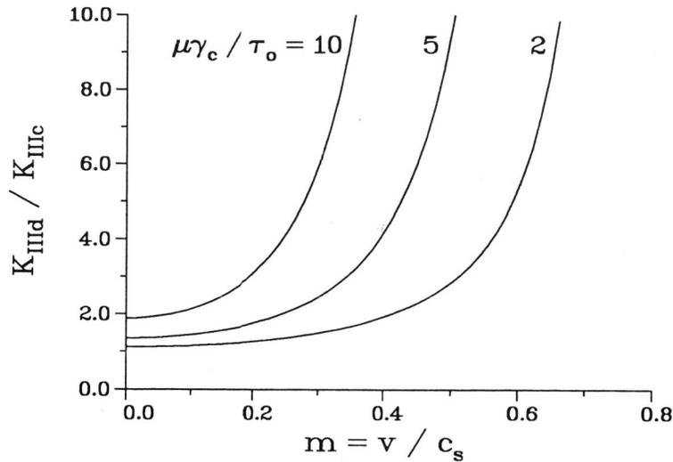
Fig. 2. Theoretical fracture toughness versus crack speed for steady growth of a mode III crack according to the critical plastic strain at a characteristic distance criterion, for three levels of critical plastic strain  $\gamma_c$  equal to 2, 5 and 10 times the yield strain  $\tau_0/\mu$ .
