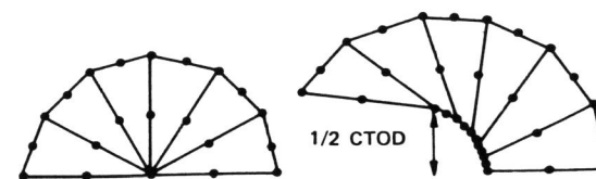
Fig. 4. Deformation of the crack tip, and definition of CTOD
