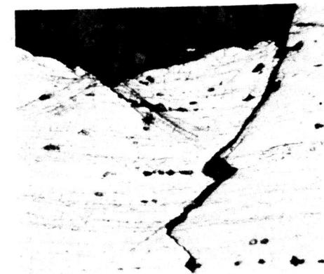
Fig.12 Ductile Fracture Initiation in As-Quenched 7010 alloy
