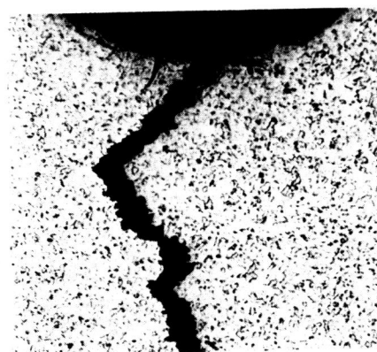
Fig.11 Ductile Fracture Initiation in Prestrained Mild Steel
