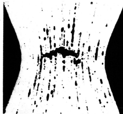
Fig.2 "Cup-cone" Fracture in a mild steel tensile specimen.
