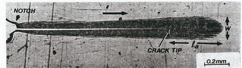
Fig. 2. Transmission optical micrograph showing a well developed CL during slow propagation. Horizontal arrow indicates the direction of propagation.
