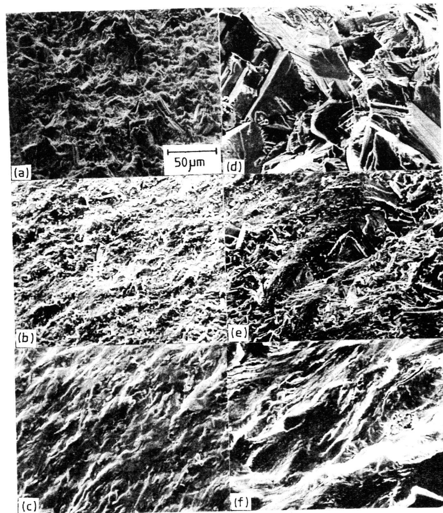
Fig. 3. Near-threshold fracture surfaces, Astroloy. Fine grain size: (a) 20^\circ\text{C} (b) 200^\circ\text{C} (c) 600^\circ\text{C} . Coarse grain size: (d) 20^\circ\text{C} (e) 200^\circ\text{C} (f) 600^\circ\text{C} .
