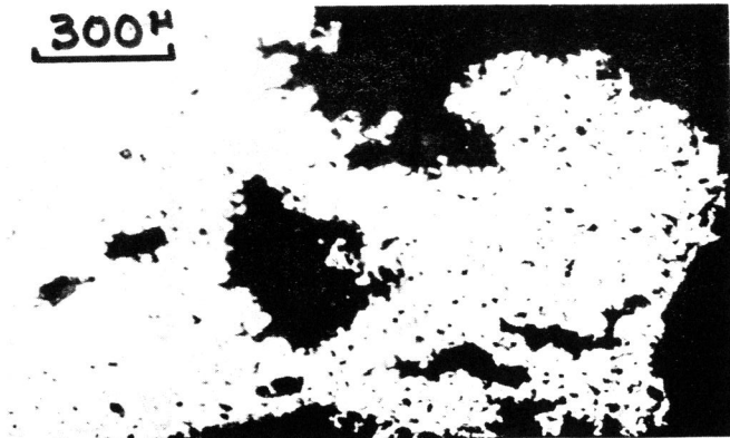
Fig. 4. Optical micrograph of the intense cavitation in 7475 Al alloy in the vicinity of fracture at a strain-rate of 5 \times 10^{-3} \text{ s}^{-1} .
