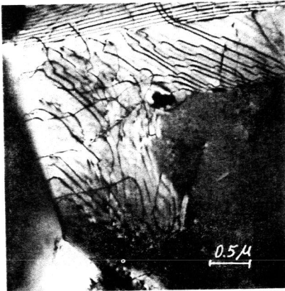
Fig. 7. Cavity at interface of particle and \alpha matrix, close to a triple-point region. (TEM X 27,500)
