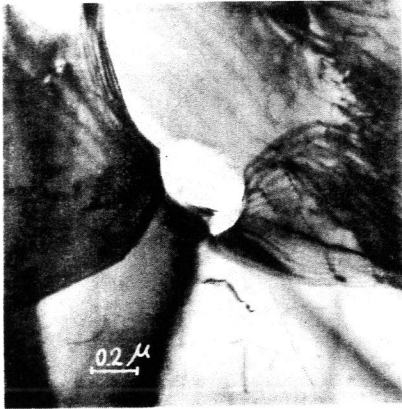
Fig. 5. Cavity at grain boundary triple point, at early strain, 800°C, 10^{-4} \text{ s}^{-1} , \epsilon = 0.2 . (TEM, X 60,000)
