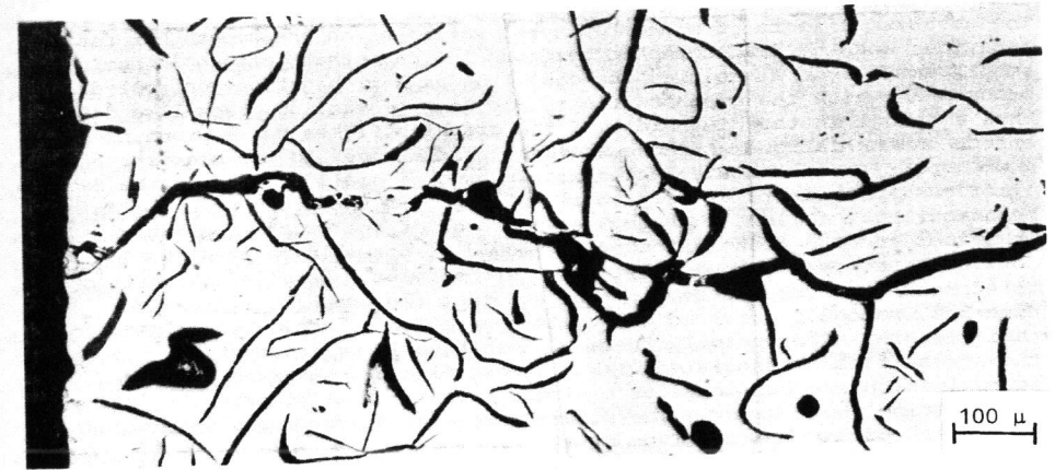
FIG. 3. Fatigue crack developing from smooth surface in flake graphite cast iron
