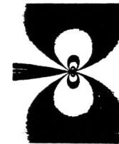
Fig. 2 Spreading of Fringes Away from Flaw Surfaces - Mode I
