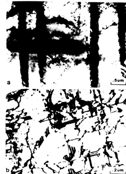
Fig. 5. Transmission electron microscopy of eroded substructure in Cu-6Al in the early stages of erosion ( 10^8 impacts at 24.7\text{ m/sec} ). a) Slip bands formed 2\text{--}5 microns below the eroded surface. b) Stacking faults and randomly oriented dislocations 5\text{--}10 microns below the eroded surface.
