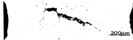
Fig. 10. Formation of the central crack in a SC2 ST plain tensile specimen.
