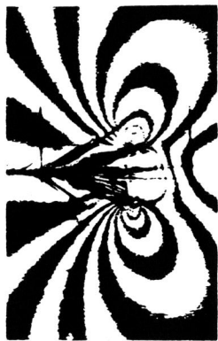
Fig. 4. Isochromatic-fringe pattern representing crack propagation after branching (courtesy of Prof. J.W. Dally).
