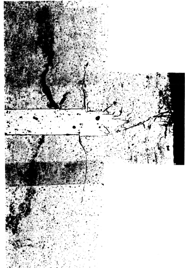
Figure 11. Appearance of an 1100 Aluminum wire marker in the rim of a 50 mm, 7075-T6 aluminum disk after N = 10^4 rolling contacts at p_0/k = 4 (Huang and Hahn, 1983).
