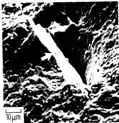
Fig. 4. Fatigue surface showing plate MnS particle
