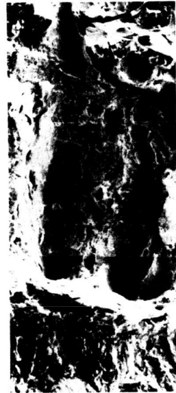
Fig. 12. Stable tearing at -25 °C (v=0.83 m/s).
