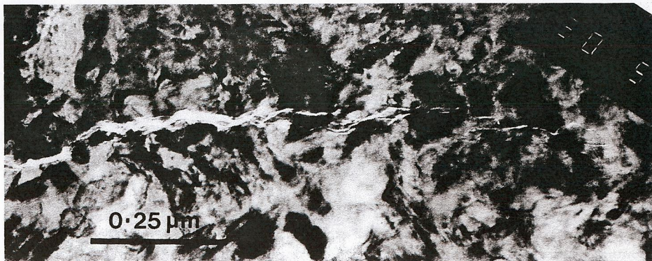
Fig. 4. Crack precipitate interaction in peak-aged 3.8 wt.% Ca-PSZ.
