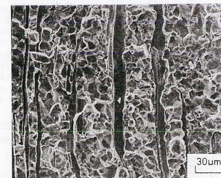
Fig.8. Fracture surface from high strength steel in SL orientation.
