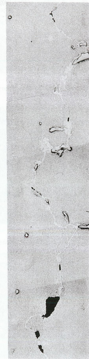
Fig. 1 x480 Cavitated grain boundary and large pore 30mm from fracture.
