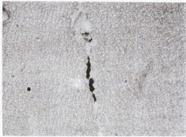
Fig. 2 x1200 Cavities remote from fracture.
