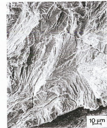
Fig. 7: Rupture surface in hydrogen at 0.15 10^{-1} MPa
