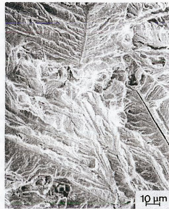
Fig. 3: Rupture surface in oxygen at 0.15 MPa
