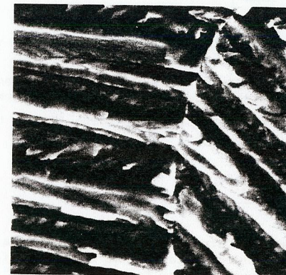
Fig. 3. Furrows formed on the fatigue fracture surface of a specimen tested in air at \Delta K \sim 16 \text{ MN m}^{-3/2} . X 6,400
