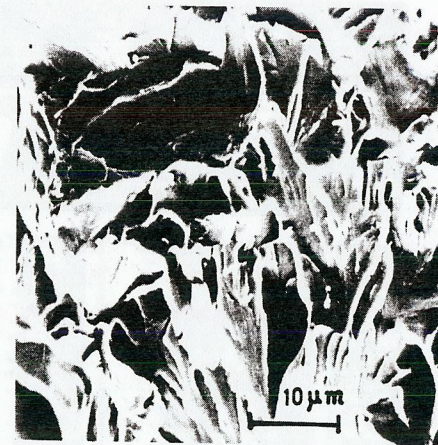
Fig.17. Quasicleavage fracture in steel PA—fractograph of MNB specimen after bending. Fig.18. Dimple fracture in steel PA-N under similar conditions, compare with Fig.17.
