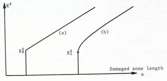
Fig. 11 Resistance curves : (a) Tearing modulus model (b) General model with increasing h.
