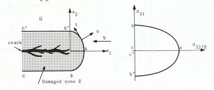
Fig. 2. (a) Steady-state moving damaged zone Z with the velocity V. The damage front is BB'.
