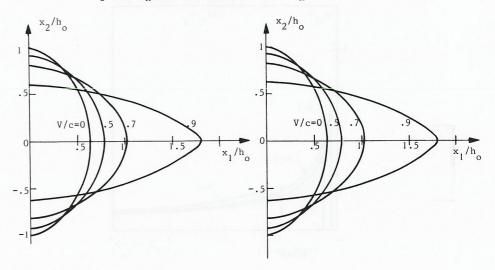
Fig. 5 Damage fronts in the small-scale damage model, with energy criterion for several velocities V/c.
