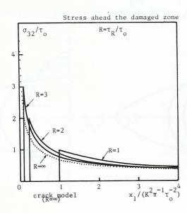
Fig. 7. Stress  $\sigma_{32}$  ahead the damage front. Singularity in the linear fracture Mechanics (dotted line,  $R = \infty$ ).
