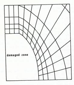
Fig. 8. Damage front in mode I by the use of a finite element method.
