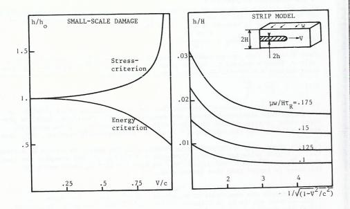
Fig. 3 Variation of h with the speed V. Stress-criterion (Constant  $K/\tau_p$ ), Energy-criterion (Const. $K_7^2\beta\tau_R^2$ ).
