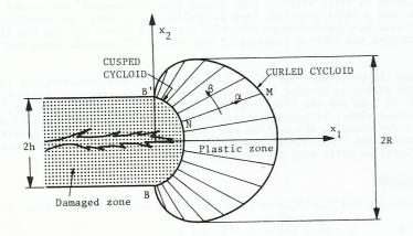
Fig. 10 Elastic, plastic and damaged zone in mode III from Bui's solution. The front is a cusped cycloid and the elastic-plastic boundary is a curled cycloid.
