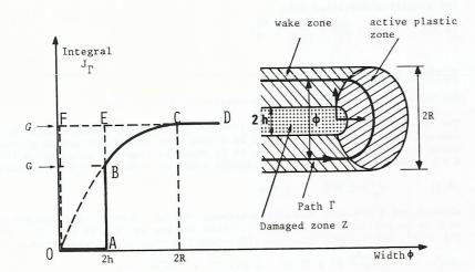
Fig. 9 Variation of the path-integral J with the width of the contour, for different models, elastic-plastic-damage OABCD, elastic-damage OAED, crack in perfect plasticity OBCD, crack in elasticity OFD. The characteristic values are G (fracture energy rate) and G (energy-release rate).
