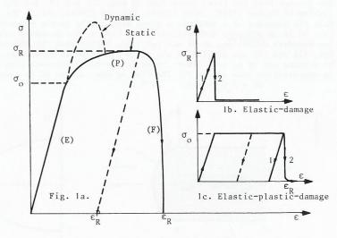
Fig.1. (a) Static and dynamic stress-strain curves.
