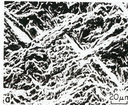
Fig. 7 Scanning electron micrograph of BQ, Ti-6Al-4V tested at -70°C, (a) no hold, (b) hold.
