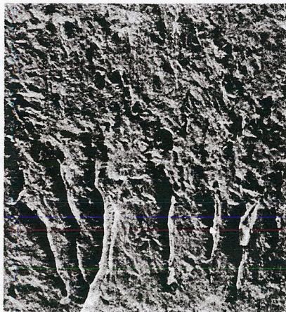
Fig. 2. 26NCDV14 Fractography (X22). From top to bottom, Mode I and Mode I+III loadings.
