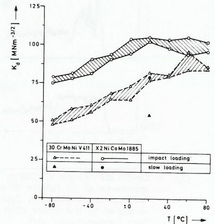
Fig. 12. Dynamic stress intensity factor vs test temperature for WOL-1X-specimens of 30 CrMoNiV 411 and of X2 NiCoMo 1885.
