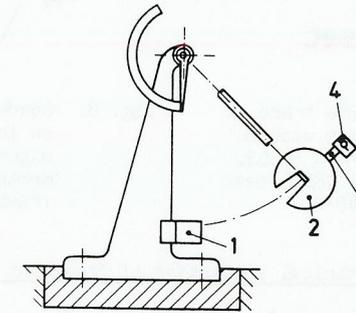
Fig. 6. Schematic of impact machine for testing WOL-1X-specimens (1 anvil, 2 hammer, 3 load cell with thread, 4 WOL-1X-specimen with cross-pin).
