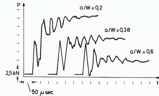
Fig. 3. Load-time traces of Charpy V-notch specimens of 22 NiMoCr 37 with various crack lengths  $a/W$ . Test temperature: 20 °C
