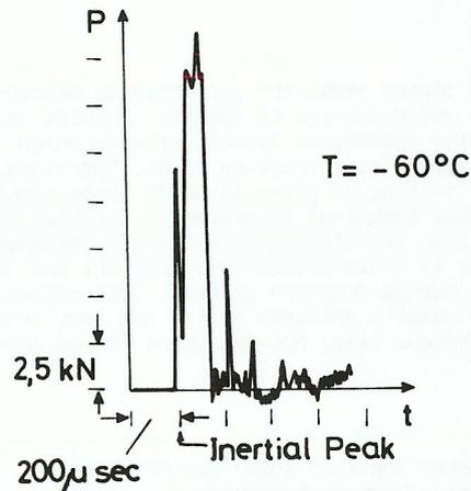
Fig. 1. Typical load-time trace of a Charpy V-notch specimen of 22 NiMoCr 37
