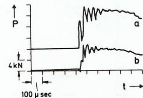
Fig. 5 Load-time signal (a) measured on tup, and strain-time signal (b) measured on instrumented Charpy V-notch specimen of 22 NiMoCr 37 at 20°C.
