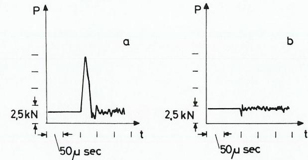
Fig. 2. Load-time traces of specimens consisting of two broken halves cemented together.
