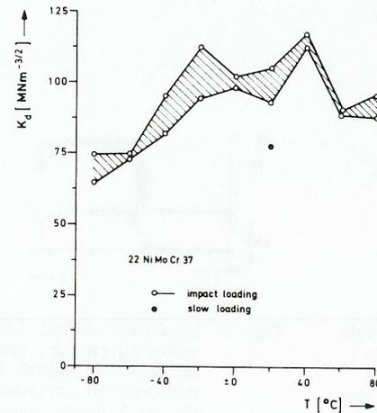
Fig. 11. Dynamic stress intensity factor vs test temperature for WOL-1X-specimens of 22 NiMoCr 37.
