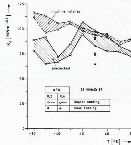
Fig. 9. Dynamic stress intensity factor vs test temperature for Charpy V-notch specimens of 22 NiMoCr 37 with and without fatigue cracks.
