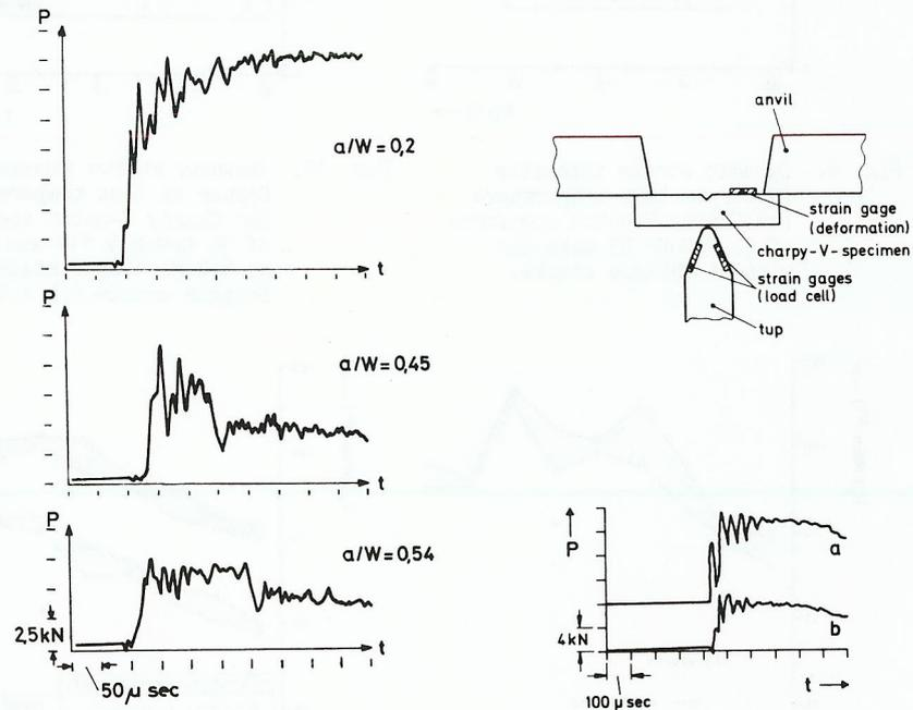
Fig. 4 Load-time traces of Charpy V-notch specimens of 22 NiMoCr 37 with various crack lengths. Specimens cemented to and moved with the tup. Test temperature: 20°C.
