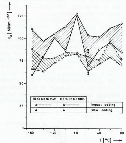
Fig. 10. Dynamic stress intensity factor vs test temperature for Charpy V-notch specimens of 30 CrMoNiV 411 and of X2 NiCoMo 1885 containing fatigue cracks  $a/W = 0,4$
