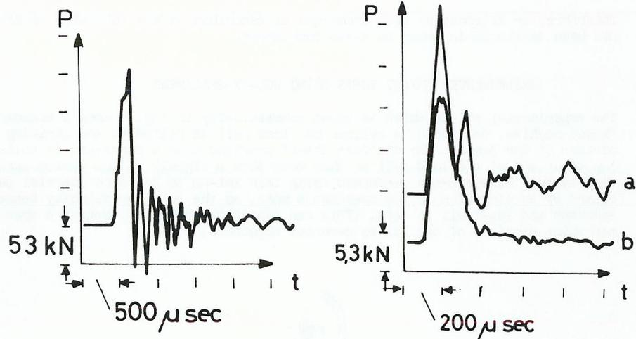
Fig. 7. Typical load-time trace of a WOL-1X-specimen with a crack length  $a/W = 0,653$ . Steel X2 NiCoMo 1885, test temperature:  $-40^{\circ}\text{C}$ .
