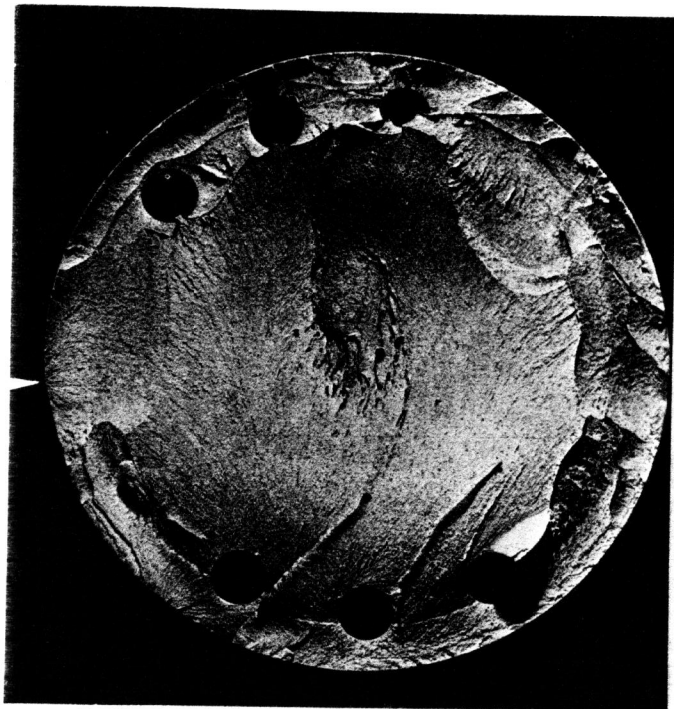
Figure 2 Fracture Surface of the Left Portion of Spindle. The Arrow Indicates an Initiation Site near the Neutral Axis in Bending
