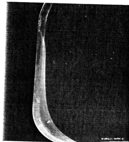
Figure 1 In Plane Cracking in an Airliner Cabin Window. Window Size Approximately 385 mm x 285 mm
