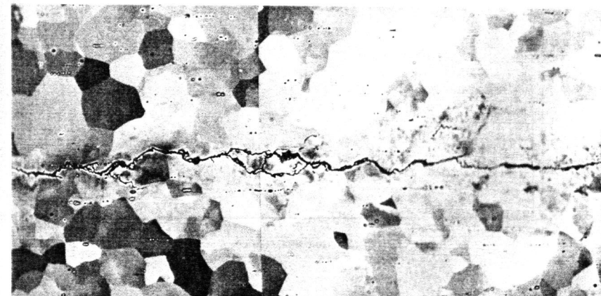
Figure 2 Fatigue Crack at \Delta K = 11 \text{ MPa}\sqrt{m} Showing the Formation of Subgrains Due in Moist Air (Left Side) and Dry Nitrogen (Right Side) Environments. Backscattered Electrons. 400X
