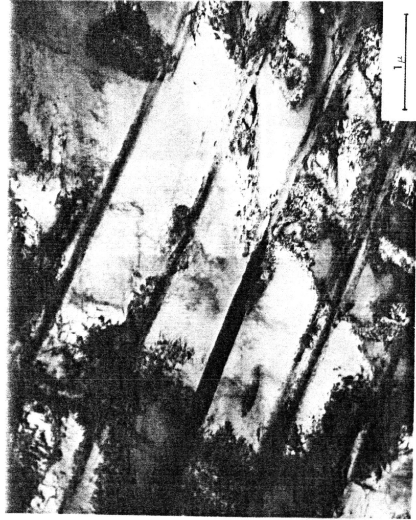
Figure 3 Deformation Twinning in Beta-III Solution Treated At 1005K and Tested At 77K
