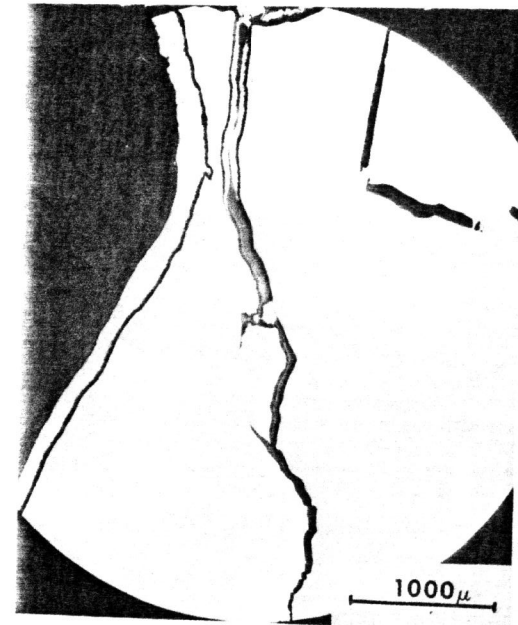
Figure 6 Illustration of Predominantly Intergranular Secondary Cracks in Beta-III Solution Treated At 1005K. RA = 60.5 pct. Test Temperature: 163K
