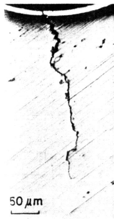
Figure 5 An Example of a Non-Propagating Crack Appearing in a Specimen with a Hole and Lines
