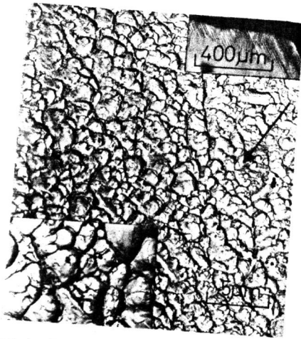
Figure 7 Fractograph (EM)* after sub-critical crack growth of Al-Zn-Mg in liquid alloy. Top insert (optical micrograph) shows deformation associated with sub-critical crack growth revealed by ageing after fracture, sectioning, polishing and etching. Bottom insert shows fractograph (EM) of critical (overload) crack growth in air (same magnification as main figure).
