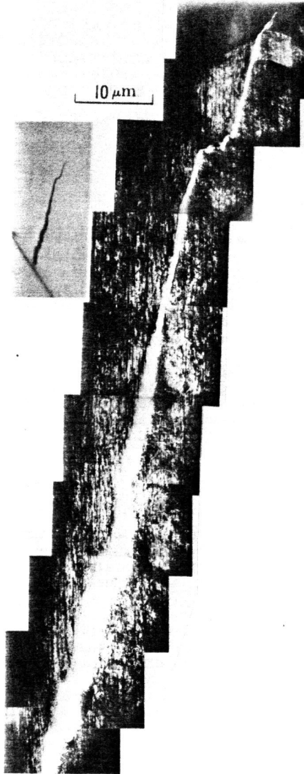
Figure 3 Dislocation structure near the sides of the crack which have grown up to the length \cong 150 \mu\text{m} .
