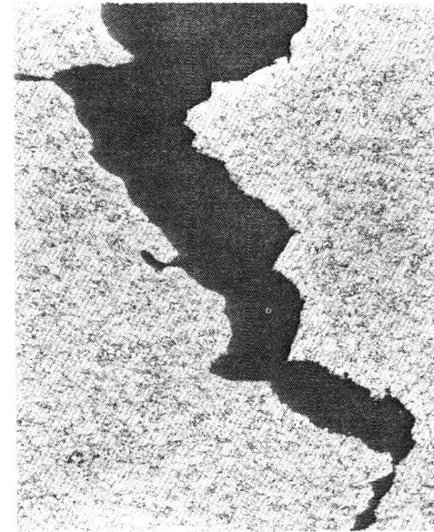
Figure 19 Zig-Zag Fracture in HY80, Prestrained 20%; After [45] X 150
