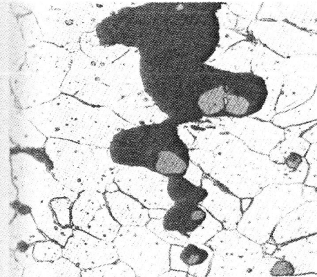
Figure 10 Fibrous Crack Growth in Free-Cutting Mild Steel (courtesy R. F. Smith) X 600
