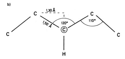
Fig. 1: Conformation of a polyethylene-chain without (a) and with (b) a radical site
