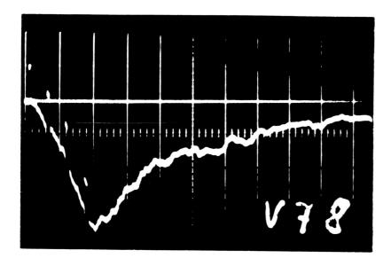
Light emission during fast crack propagation in glass
