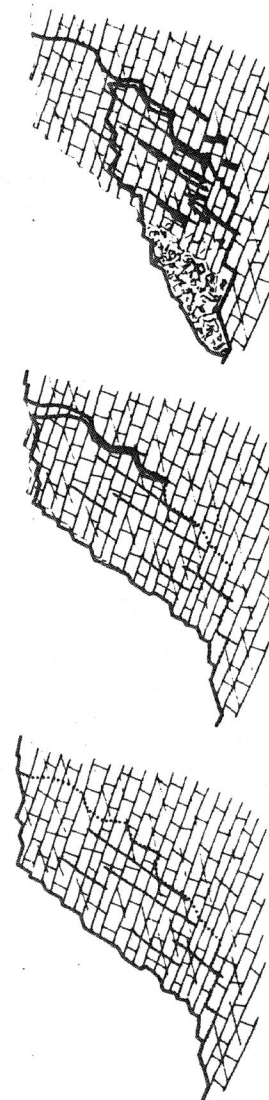
FIG.1 PROGRESSIVE FAILURE IN ROCK
