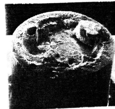
Fig.5 Nitrided push-pull specimen fractured at \pm 66.5 hbar
