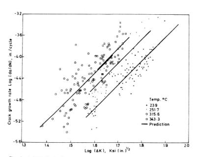
Fig.: 2. A-212B Steel effect of temperature.
