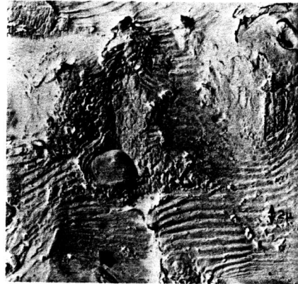
Fig. 9. Static growth at inclusions in 7075-T6 at fatigue crack growth rate of 1 micron per cycle.
