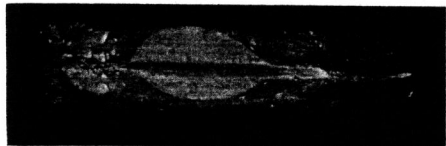
Fig. 3. Failure from elongated defect. Note propagation in minor axis direction.
