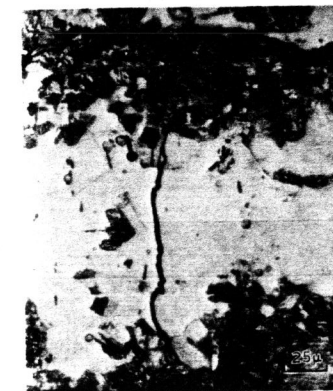
Fig. 9. \sigma = 28 \text{ kg/mm}^2 , N = 10^7 the crack, impeded its propagation by surrounding microstructures (non-propagating crack) after light electro-
