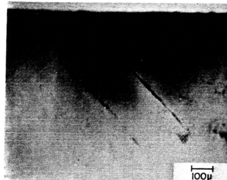
Fig. 11. Void accumulation and crack nucleation at kink boundaries in crystal at 510°C at a strain amplitude of 0.36% after 10^5 cycles.
