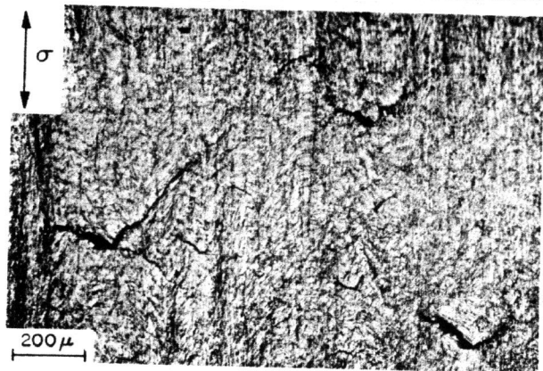
Fig. 12. Same specimen as Fig. 10 after 500 cycles showing the high density and severity of the cracks formed ( N_f = 706 cycles).
