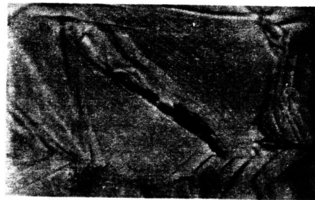
Fig. 2. In-plane hydride crack formed in a hydride platelet which had previously exhibited transverse cracking. (0.18 mm. grain size, 50 ppm. hydrogen, test temperature -196^{\circ}\text{C} ). \times 315 .
