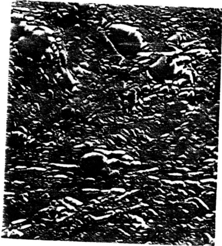
Fig. 2. Steel 81M double-quenched-and-tempered, last temper at 450C.
